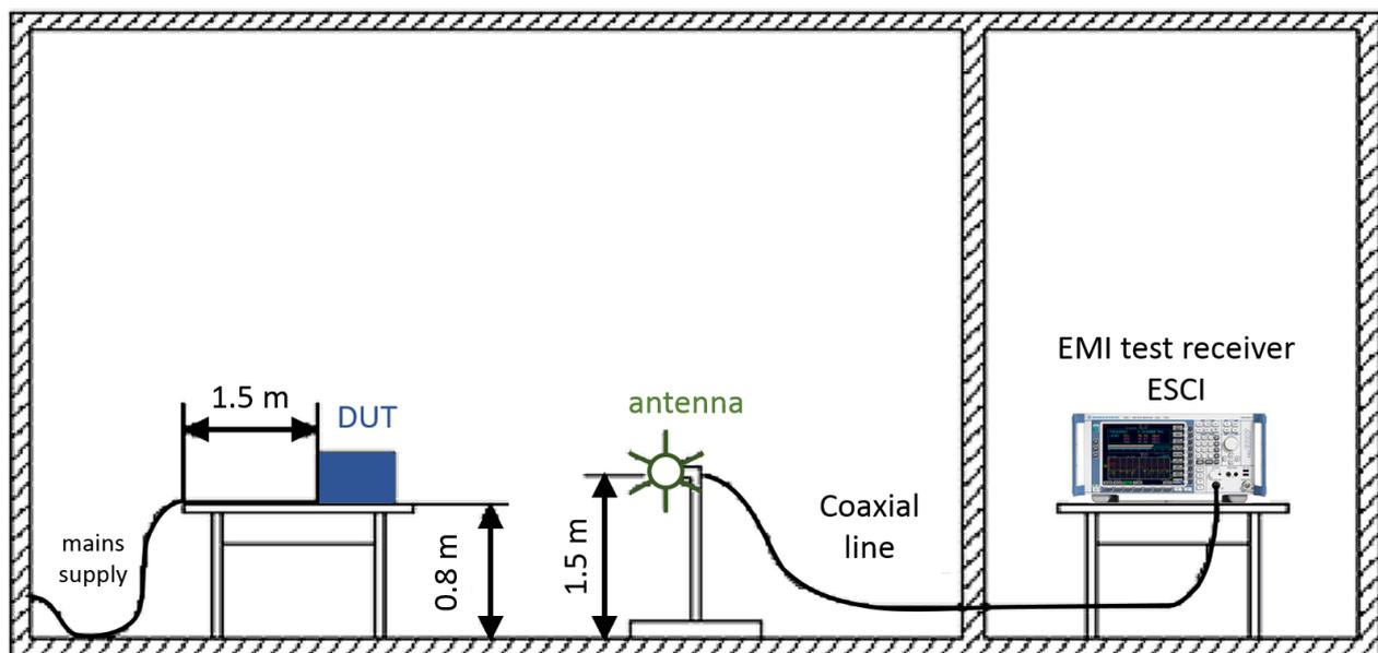
Figure 1 – Test setup in SAC (absorber pyramids not depicted)
