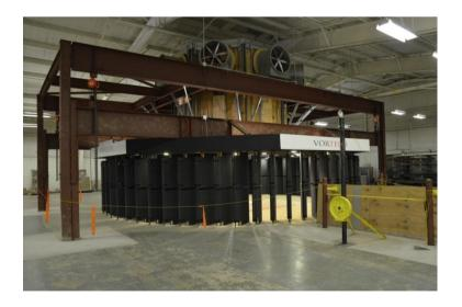
To test how much damage pieces of buildings can do to walls of save rooms they use a canon, which can shoot with much pressure huge pieces of wood. The operator told us that even discovery channel with the show myth busters did some season in this laboratories.
