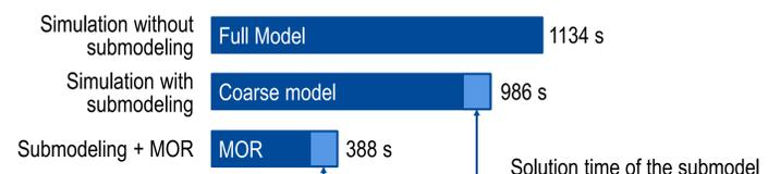
Fig.8: Computational time comparison between the thermal simulations of detailed TEG in submodel and global model. (16x Intel® Xeon® CPU E5-2687W v4 @ 3.00 GHz, RAM 324 GB, VGA NVIDIA Tesla M10)
