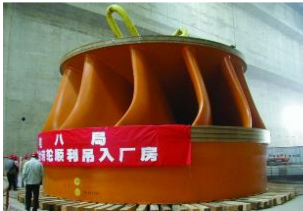
©Voith Siemens Hydro Power Generation: Sanxia_Runner04_300.jpg; Runner of a Francis turbine used for the Sanxia (Three Gorges Dam) power plant, China.; GFDL 1.2; 2003
