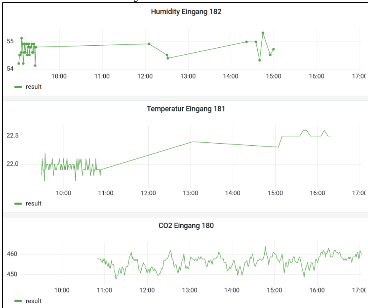
Figure 4: Gaps in the plots of temperature, humidity, and CO2 sensor values, all from the same KNX device
