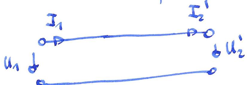
$$\Rightarrow I_2' = I_1 = \frac{I_2}{t} \Rightarrow \frac{I_2}{I_1} = t \quad (13)$$
